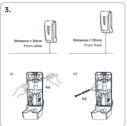
Install the dispenser on the recommended height from floor or
